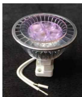
Figure 8. A 7-watt LED cup light covered with a combined filter.
