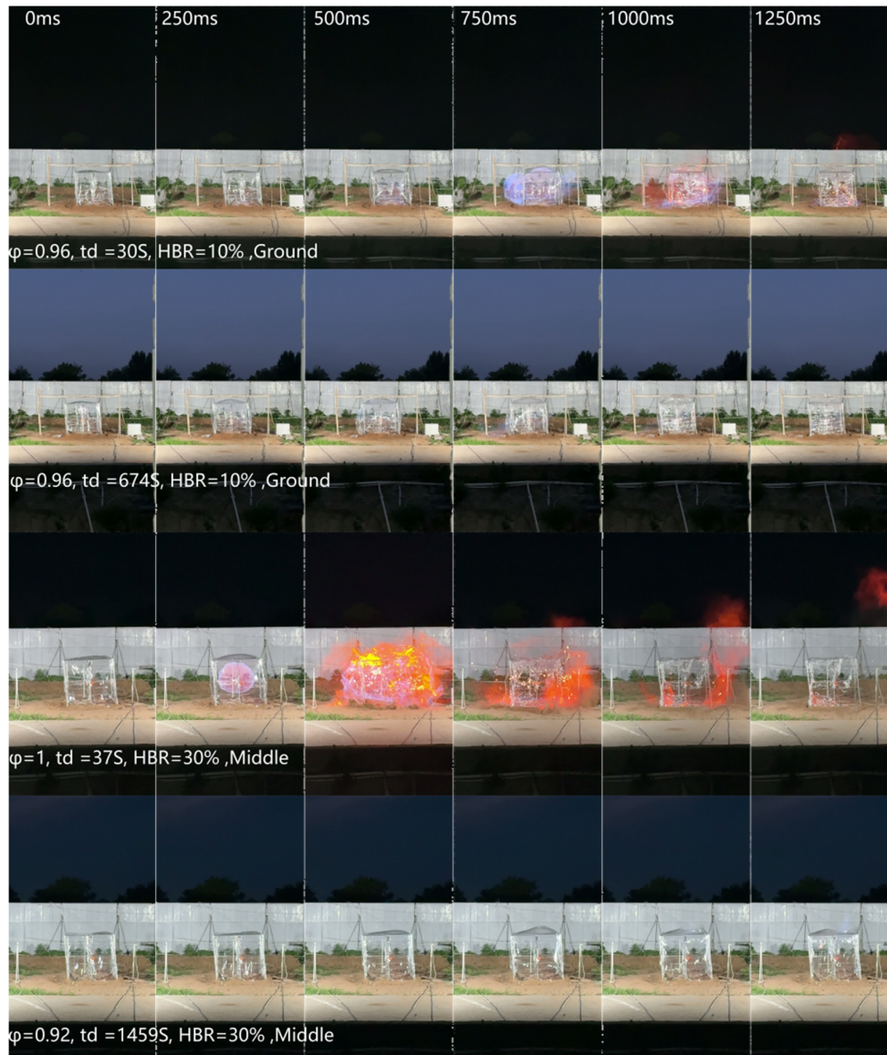
Figure 3. Flame evolution for representative cases from 0 to 1250 ms.
