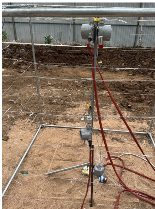
Figure 2. Arrangement of thermocouples along the central axis.
