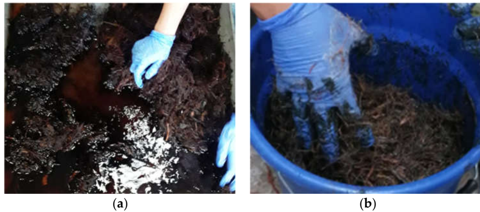
Figure 1. (a) Appearance of fibers during NaOH treatment, and (b) silica-fume treatment.
