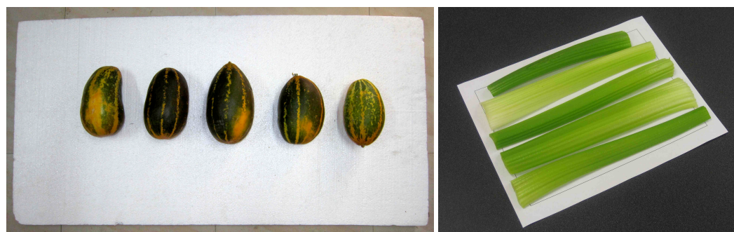
Figure 3. Images captured using a digital camera with good contrast background and reference frame (left: snap melon on thermocol board - 1.0 m × 0.5 m; right: celery on letter paper (US) with a drawn rectangle of 242 mm × 178 mm).
