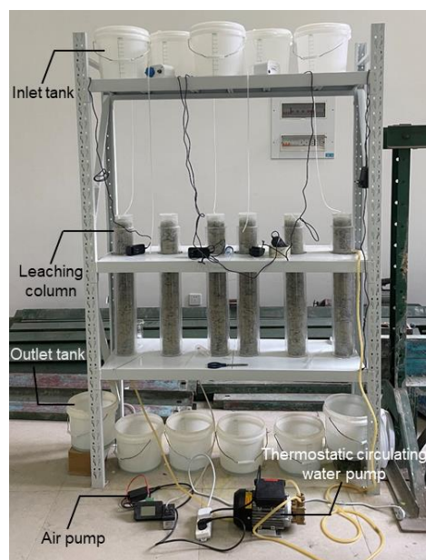
Figure 1. Airtight column bioleaching system.
