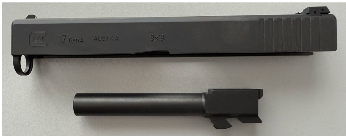
Figure 15. Slide and barrel of the Glock 17 Gen 4.
