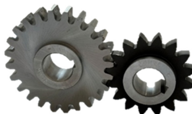
Figure 1. Test FZG gear pair, type A10, the pinion coated with W-DLC/CrN.
