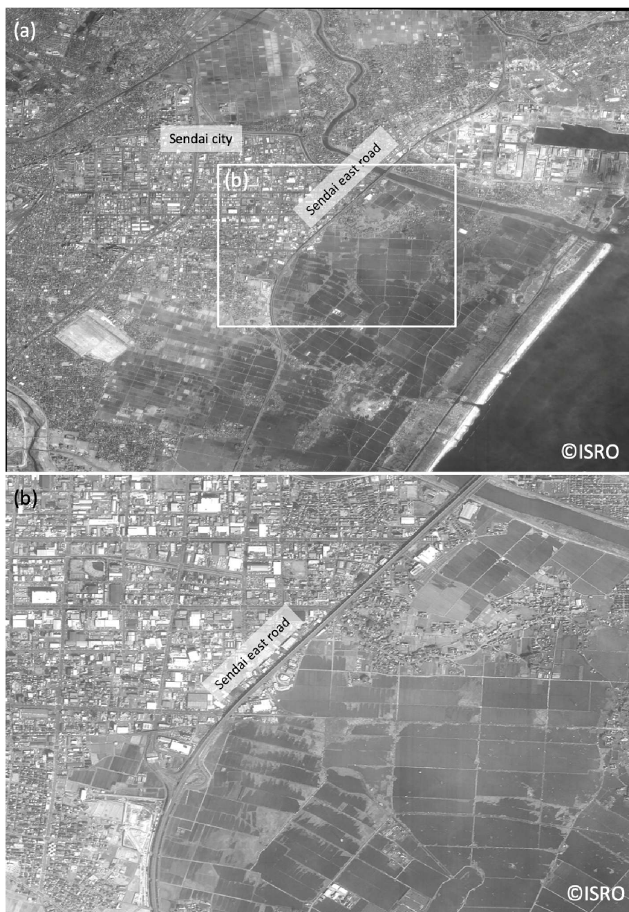
Figure 21. CARTOSAT-2 (a spatial resolution of less than 1 m and a 9.6-km swath width) image observed on March 14, 2011, over Sendai area, provided by ISRO in the framework of SA. Sendai East Road worked as a dike. Dark areas indicate flooding by the tsunami. The embankment at Sendai East Road, about 5–6 m high, parallel to and a few kilometers away from the coastal line, had been effective in stopping tsunami waves from flowing further inland. Source: SA Step-3 website.
