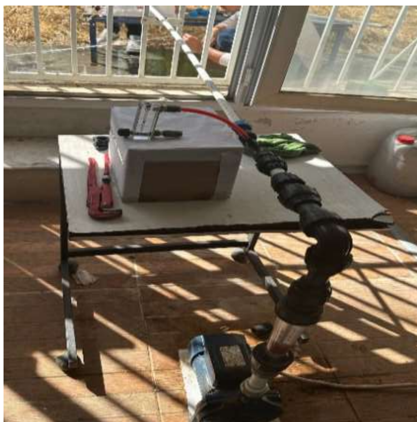
Figure 2. Test setup (Pump, water flow meter, air flow meter, Venturi device and manifold).
