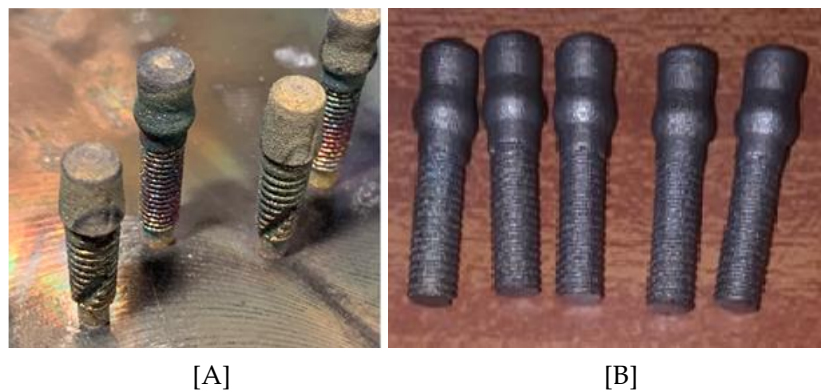
Figure 5: [A] Showing 3D-printed Dental implants before heat-treatment, [B] Showing 3D-printed Dental implants after heat-treatment. The heat treatment were performed for 2 hours hold at 800 °C in protective Argon atmosphere.
