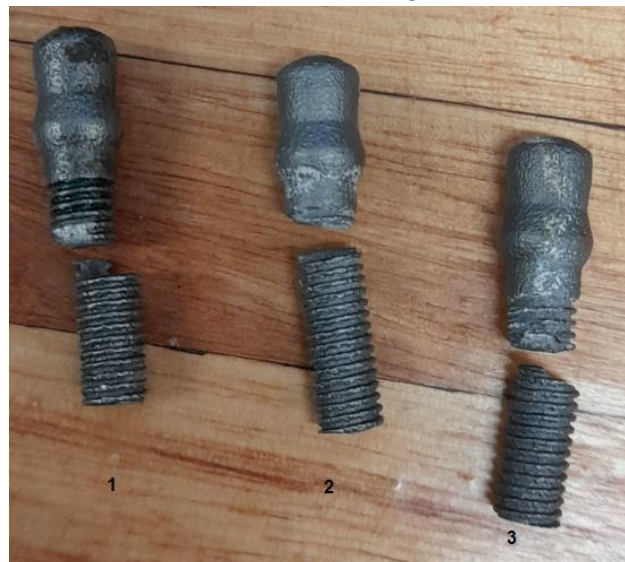
Figure 10: Fractured 3D-printed dental implants after experimental study according to ISO 14801 standard's fatigue test.
