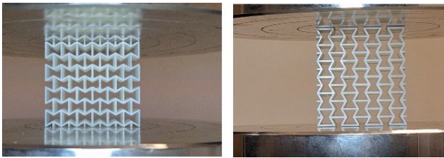
Figure 4. Placement of the specimens on the directions of X' (left) and Y' (right) on the compression test apparatus plate.
