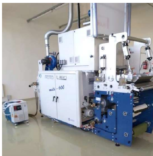
Figure 5. Pilot continuous coating and laminating machine ROTOLAB Multi 600.
