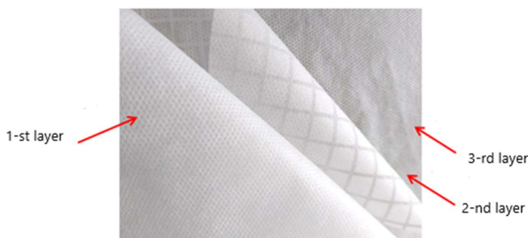
Figure 7. The arrangement of 1st, 2nd and 3rd layers of non-woven PP material in layout M890.
