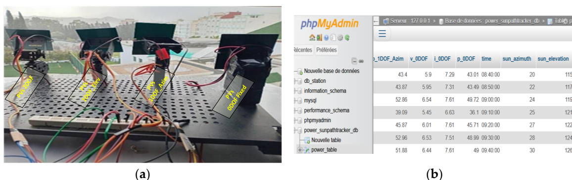
Figure 4. Some hardware and software tools: (a) Three SPT systems and fixed PVs; (b) Local database power_sunpathtracker_db.
