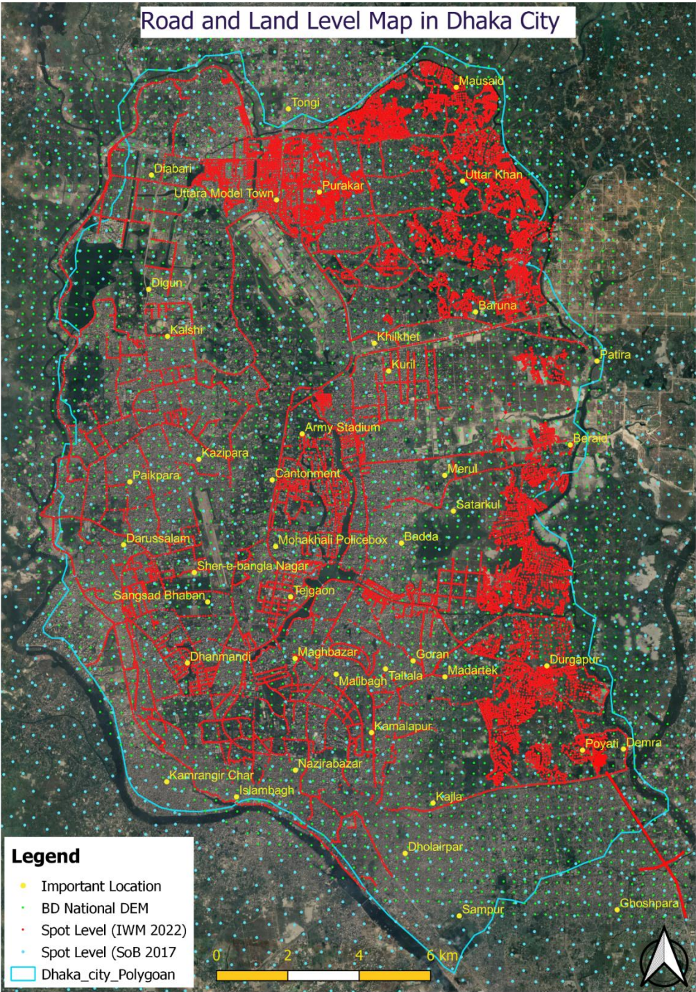
Figure 4. Spot level and road level survey for updating exiting DEM data for floodplain modelling.
