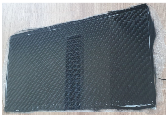
Figure 1. Photograph of a composite carbon fiber and epoxy resin test plate with embedded FBG sensors.
