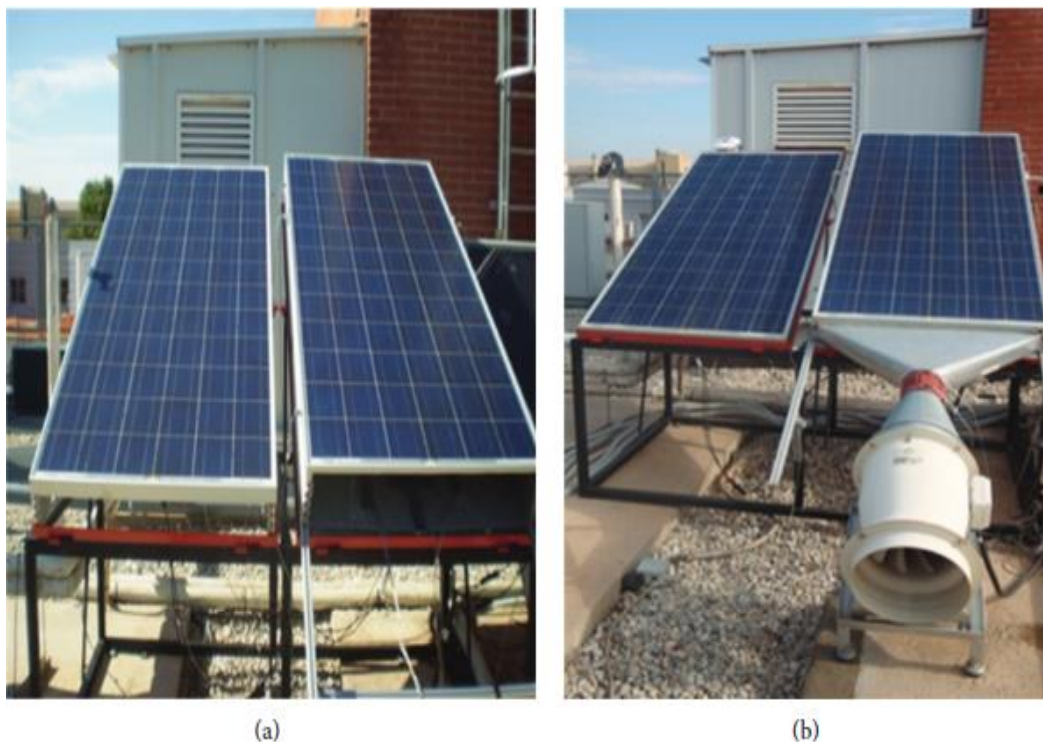
Figure 11. Solar experimental facility. The left panel labelled as panel A is not modified and the right panel labelled as panel B is above a steel plate, creating an air channel underneath it. (a) Natural convection configuration. (b) Forced convection configuration [14].
