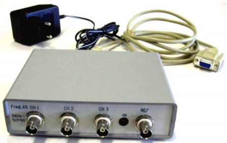
Figure A9. The appearance of the frequency meter developed and implemented in the experiment.
