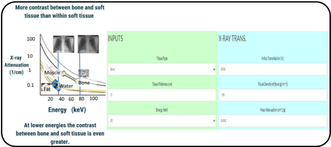
Figure 3. Influence of the X-ray attenuation vs. energy emitted in the contrast between different materials. The figure was adapted from [12].
