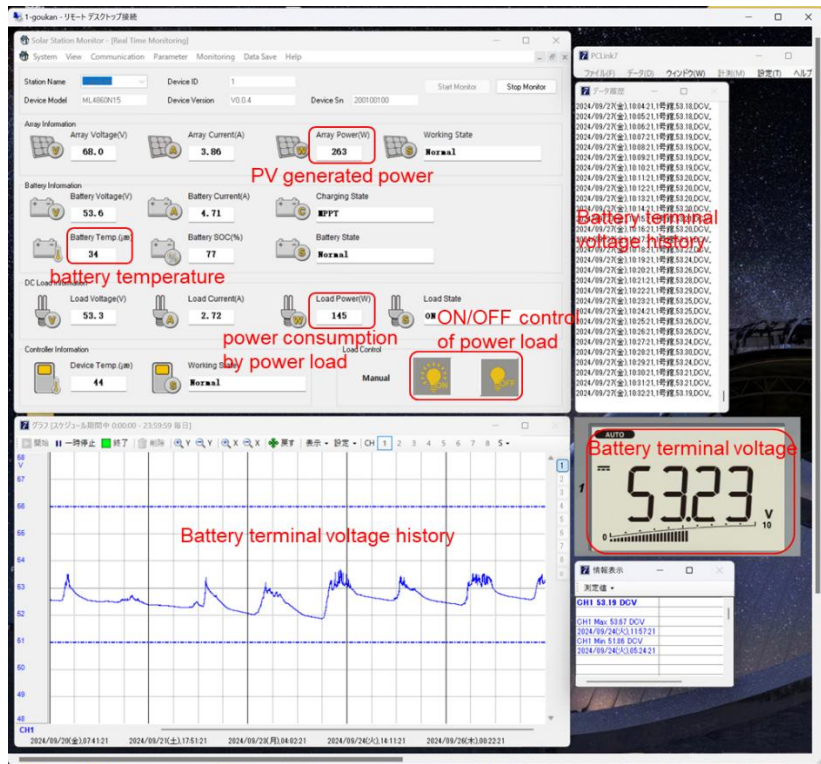
Figure 7. Monitor screen of the microgrid operation.
