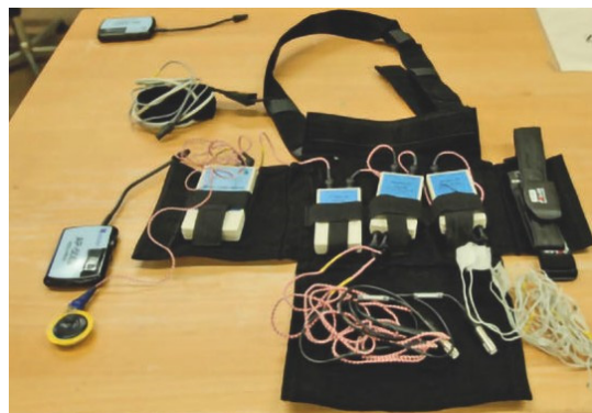
Figure 1. Fieldable mobile physiological laboratory (mobPhysioLab®) used in the studies mentioned above. Source: Wehrwissenschaftliches Institut für Schutztechnologien (WIS) – ABC-Schutz [Bundeswehr Research Institute for Protective Technologies and Chemical, Biological, Radiological, and Nuclear Protection], Munster.
