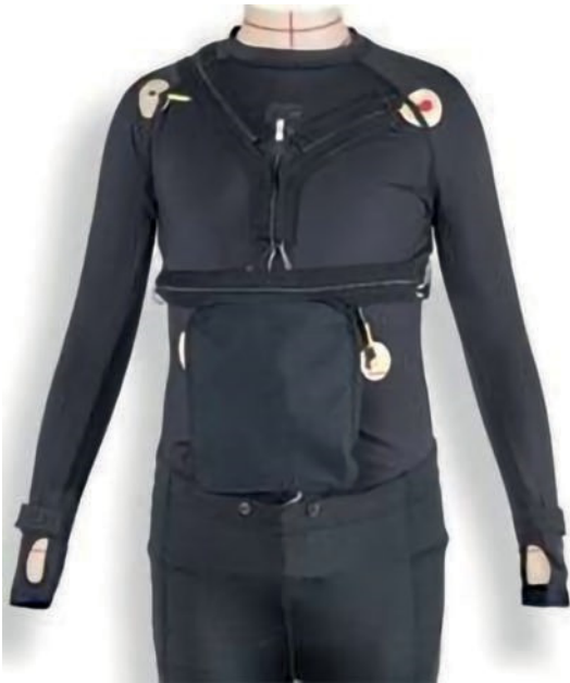
Figure 3. Prototype of a sensor suite (smart textile) used for recording skin temperature at the extremities, skin moisture, respiration rate, and heart rate. Source: Wehrwissenschaftliches Institut für Werk- und Betriebsstoffe (WIWeb) [Bundeswehr Research Institute for Materials, Fuels, and Lubricants], Erding.
