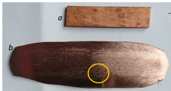
Figure 6. Photographs of the sample: (a) before and (b) after the adaptive HPS process. The circle in image (b) indicates the area in which the microstructural study was conducted. The microhardness in this area was approximately 200 HV.
