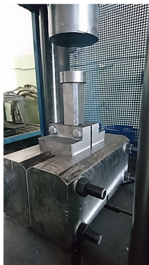
Figure 3. Photo of the adaptive HPS process rig employed.
