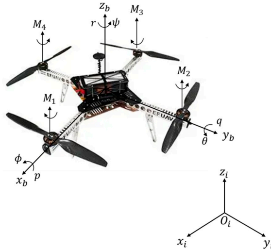
Figure 1. Attitude motion of the quadrotor in coordinate frames.
