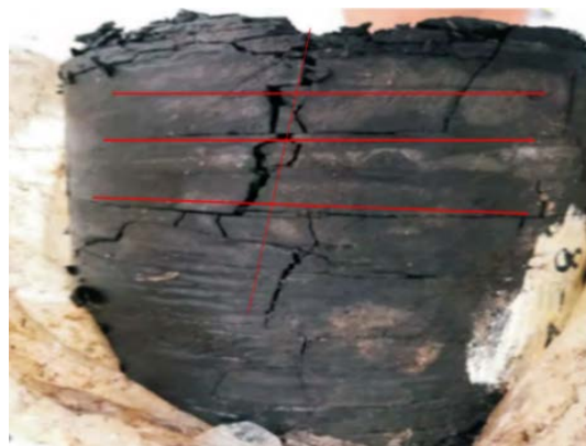
Figure 1. Image of the post-fractured fractures network in the Gulong Shale.
