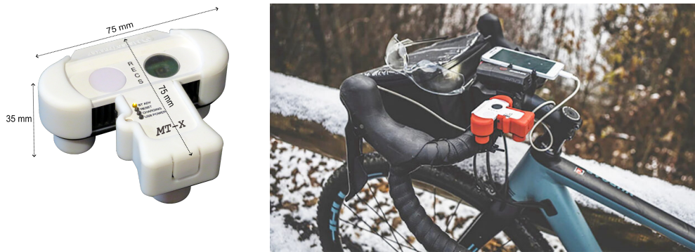
Figure 1. The Meteotracker device (on the left) and an example of installation on board of a bicycle (on the right).
