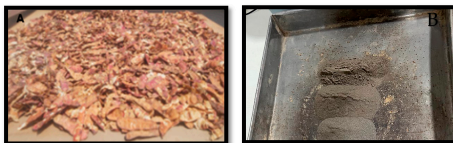
Figure 1. (A) Dried tara husk collected and selected as the base material for ash production. (B) Sample of tara ash obtained after calcination, ready to be sieved and used as an additive in the concrete mix design.
