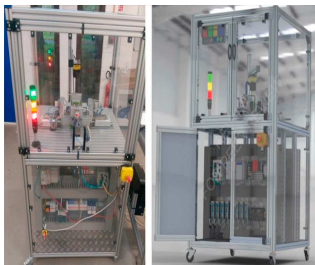
Figure 12. Physical manufacturing cell (a) and its virtual equivalent (b) [122].
