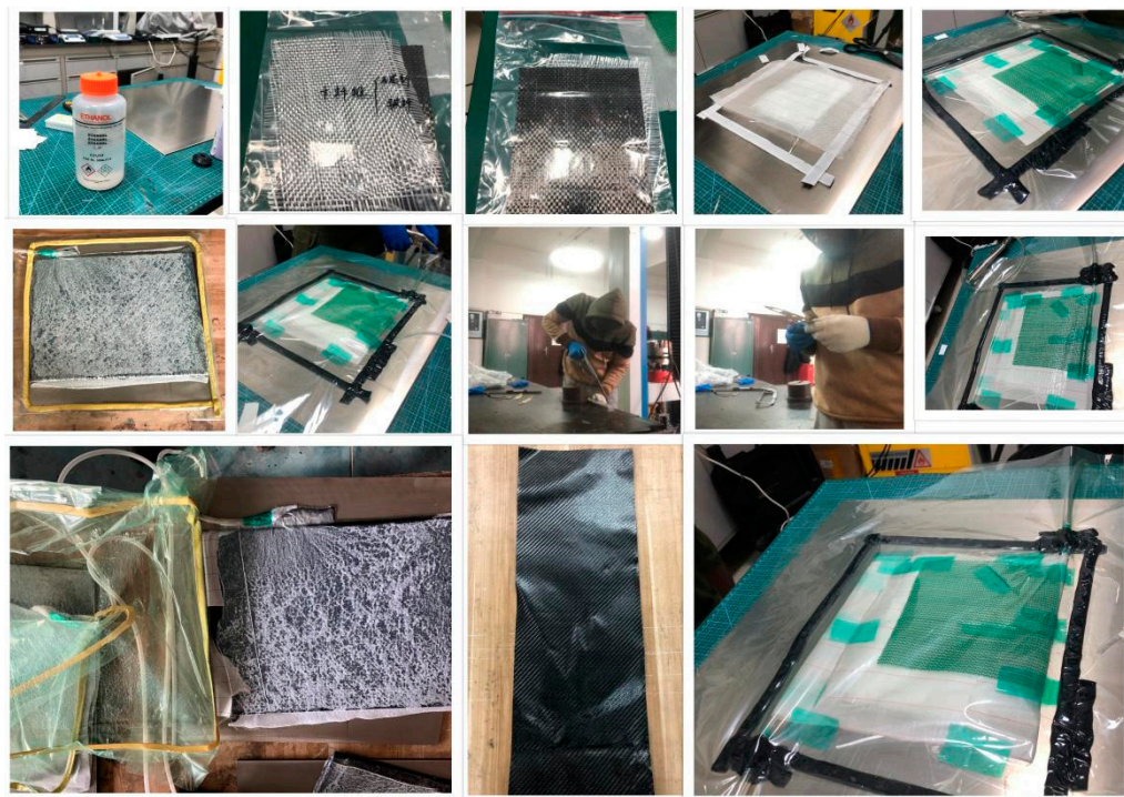
Figure 11. Composite skin fabrication using vacuum moulding process.
