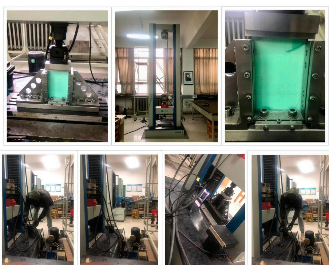
Figure 4. Experimental compression test setups (specimen, fixture, and antesting machine).
