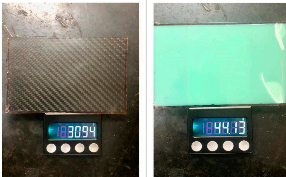
Figure 10. Composite plates mass after compression test.
