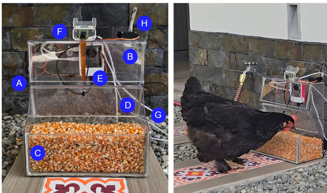
Figure 4. Functional prototype of the AVITRÓN system. (a) Front view of the assembled device showing the main components: (A) acrylic structure, (B) internal control module, (C) feed compartment, (D) dispensing gate, (E) Raspberry Pi 5, (F) AI camera, (G) support base, and (H) MG996R servomotor. (b) Experimental validation in a real environment with a hen accessing the system during selective feed dispensing. Dimensions: 350 × 300 × 150 mm.
