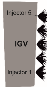
Figure 6. Calculated parcel trajectories originating from the injectors behind the IGV.
