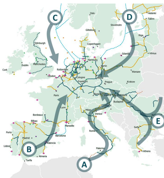
Figure 12. The five EU planned corridors for hydrogen import (source: [63]).
