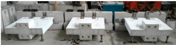
Figure 3. Finished product diagram of end hysteresis test specimen.
