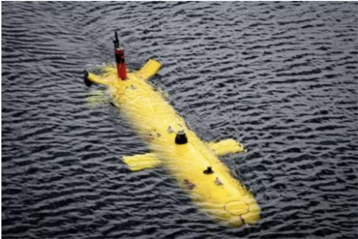
Figure 2. Explorer AUV of Memorial University of Newfoundland Sourced from[24]
