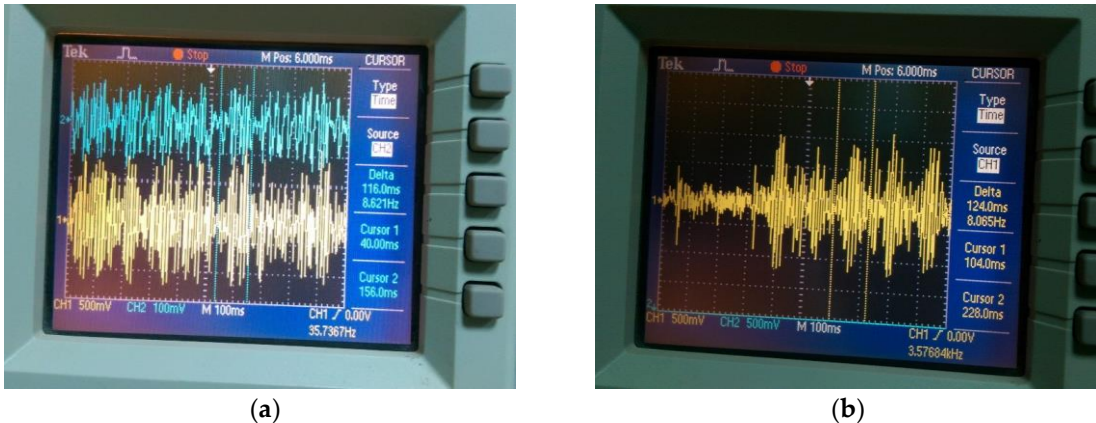
Figure 19. Observations of GMSP Simulation observed from Tektronix 2014 Oscilloscope as (a) R-Wave with 16.03mm Wavelength at 35.73 Hz; and (b) L-Wave with 1.7mm wavelength at 78.092 Hz.
