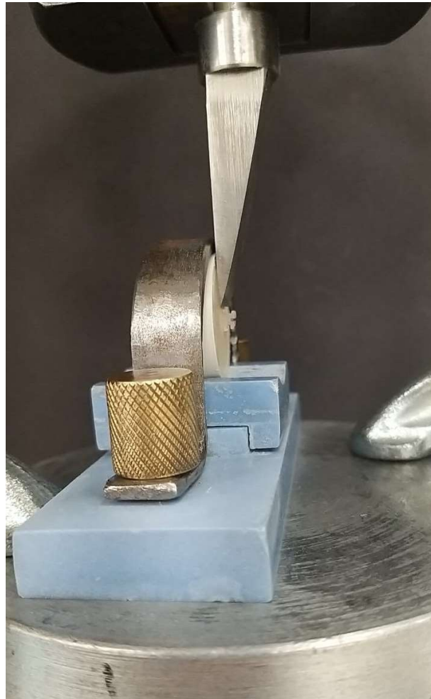
Figure 2. A sample was mounted on the universal testing machine and being subjected to shear bond strength test.
