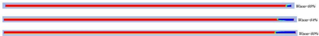
Figure 17. Contours of water vapor with different W_{vap} in capillary condensation ( T_{in}=362.17K ; T_{cool}=323K ; U_{in}=0.3m/s ; t=3.2s ).
