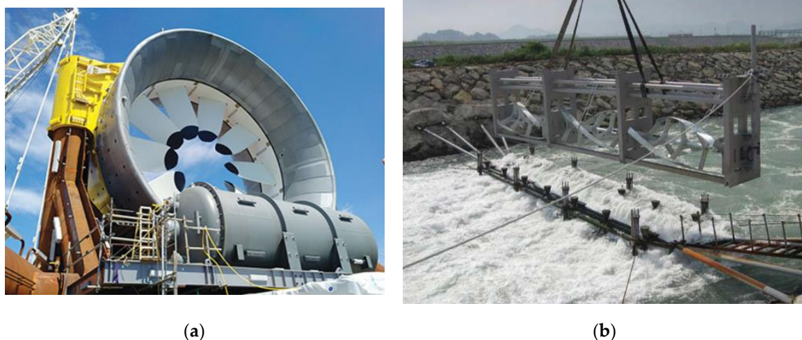
Figure 1. Large scale electricity generator installations: (a) 2 MW turbine with a permanent magnet ring generator [15]; (b) Gorlov turbine as a horizontal-axis river turbine [7].
