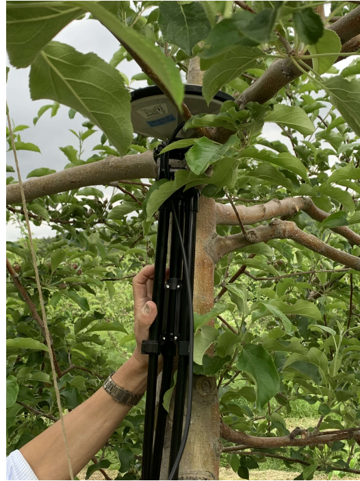
Figure 3. Installation of antennas for the acquisition of standing tree locations
