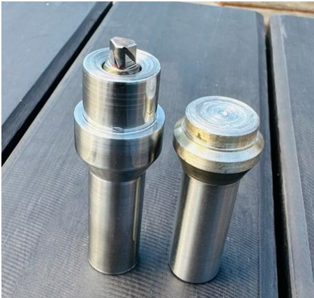
Figure 1. Pin less tool and Pin with tool utilised during the fabrication process.
