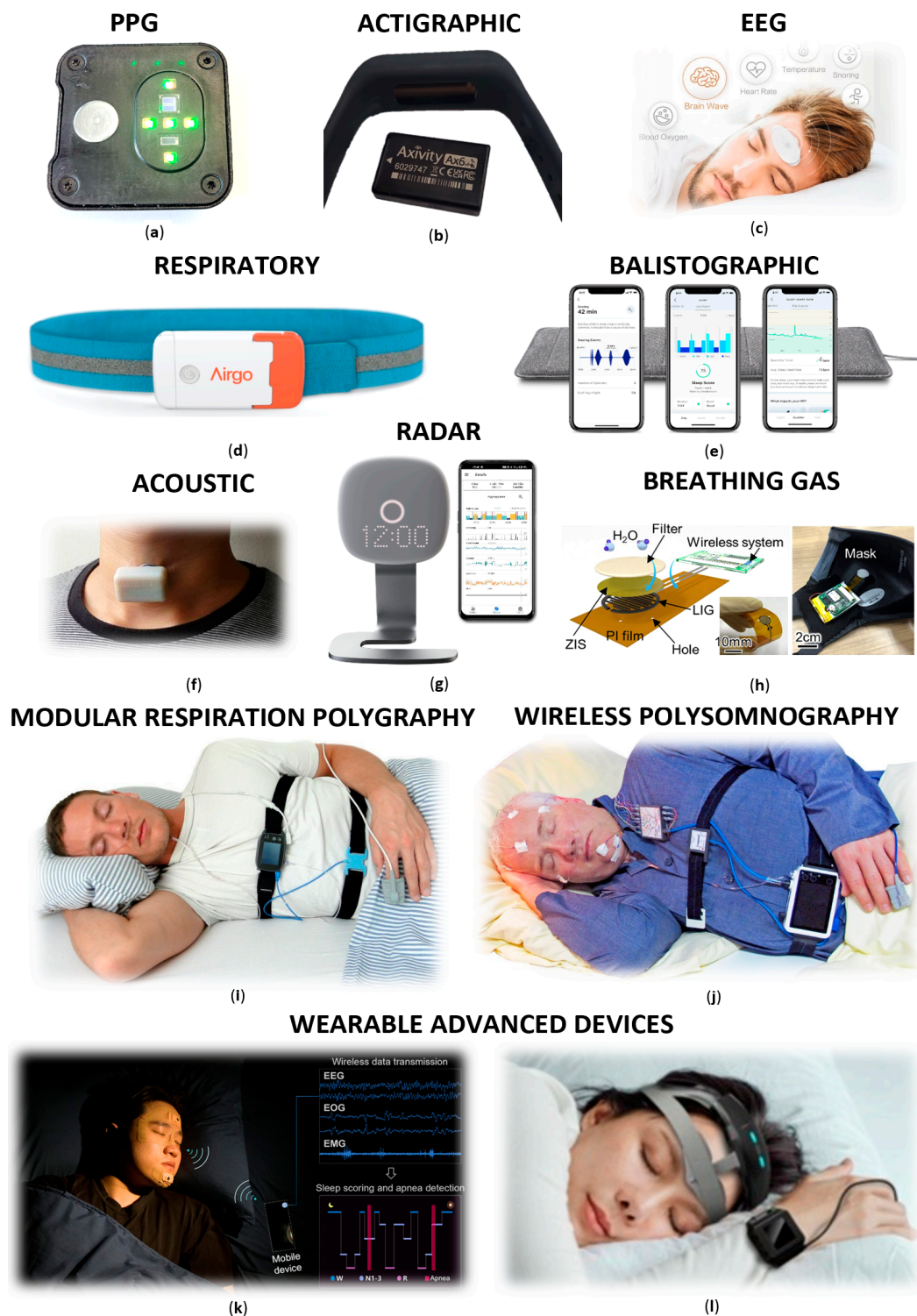
Figure 1. Sleep monitoring devices: (a) ePPG—own designed multisensor with PPG, temperature and movement sensors for sleep analysis [10]; (b) SleepActa actigraphic monitor with Dormi algorithm [101]; (c) UMindSleep EEG based sleep tracker. Reprinted from ref. [102]; (d) Airgo chestbelt for sleep respiration disorders monitoring. Reprinted from ref. [103]; (e) Withing sleep analyser based on BCG placed under bed mattress. Reprinted from ref. [104]; (f) Wearable apnoea detection device. Reprinted from ref. [105]; (g) Somnify—radar system for contactless analysis of sleep stage and RR. Reprinted from ref. [106]; (h) Flexible humidity sensor in facemask for sleep apnoea monitoring. Reprinted from ref. [107]; (i) Modular respiratory polygraphy device SOMNOtouch™ Resp. Reprinted from ref. [108]; (j) Wireless PSG device SOMNO HD. Reprinted from ref. [109]; (k) Wireless wearable sleep monitoring patches. Reprinted from ref. [110]; (l) Advanced wearable headband and wrist device WPSG-I. Reprinted from ref. [111].
