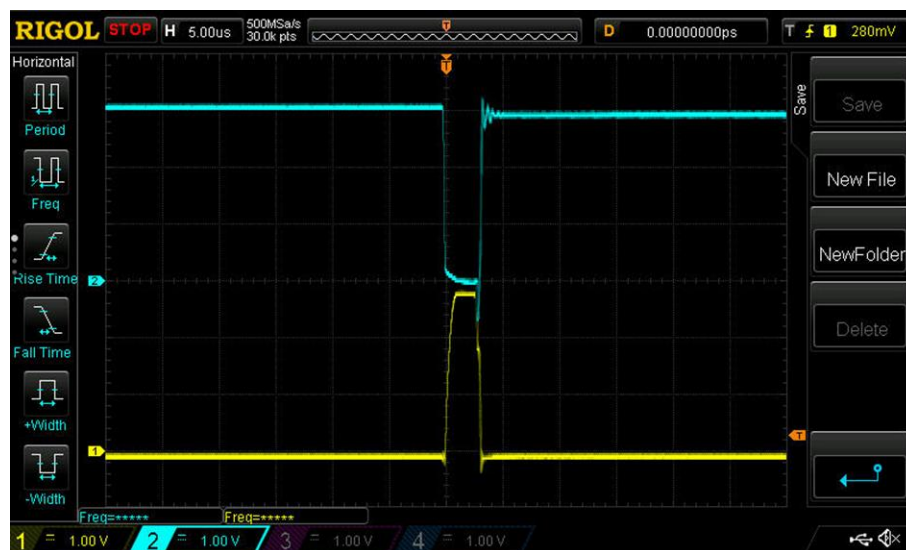
Figure 3. CH1 – the impulse of the lower transistor, CH2 – the voltage at point A.
