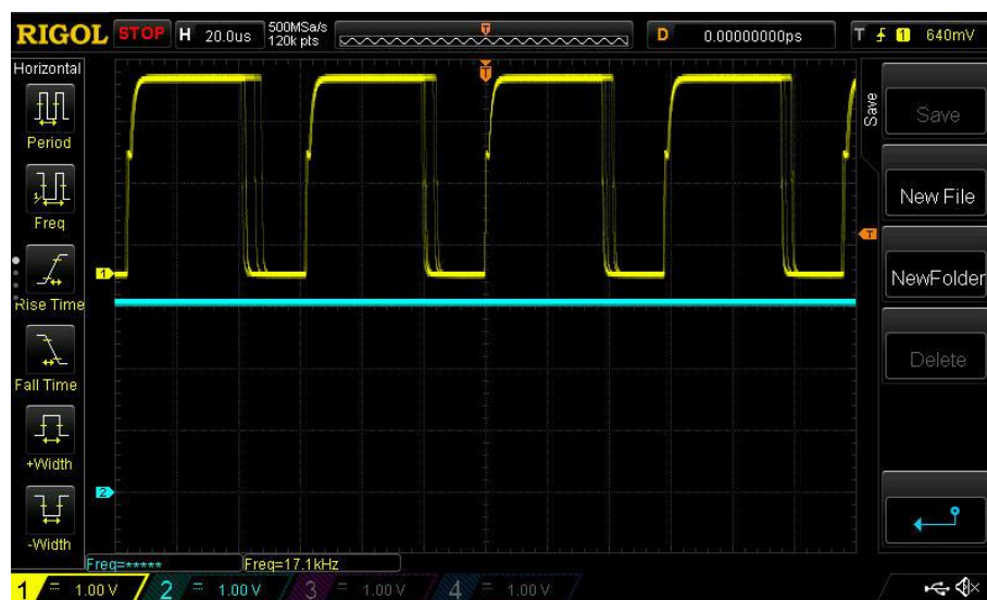
Figure 14. CH1 - the control pulses of the lower transistor, below them CN2 - the supply voltage.
