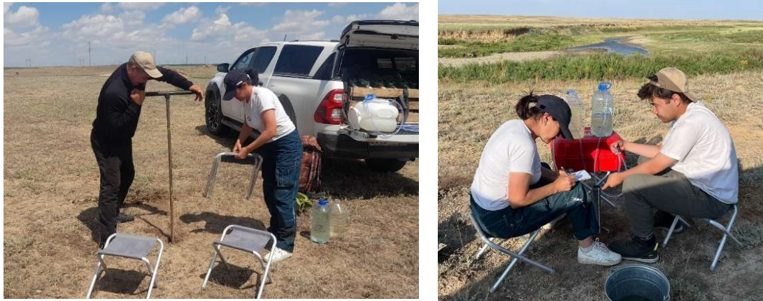
Figure 14. Field experiments for determining soil infiltration properties using in situ infiltration methods.
