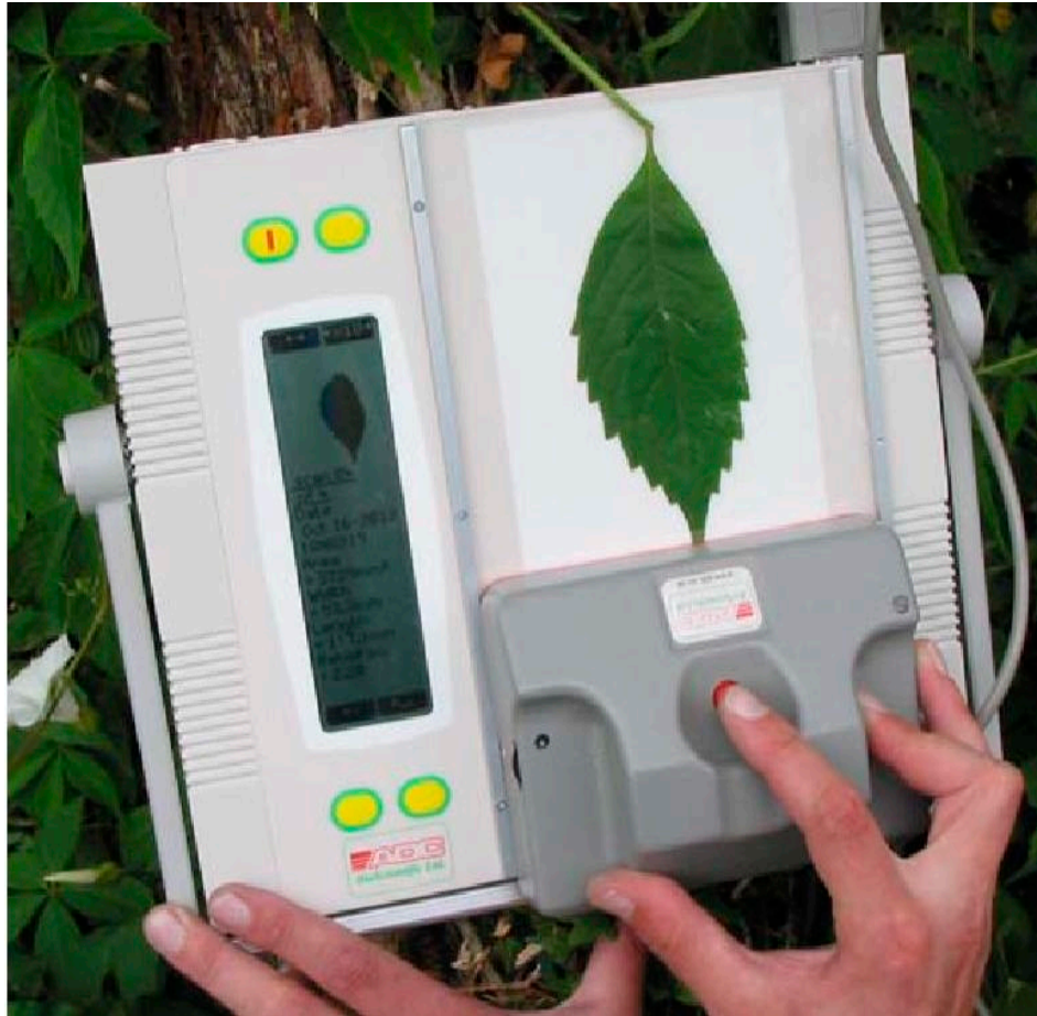
Figure 3. Leaf area determination device used during the research.
