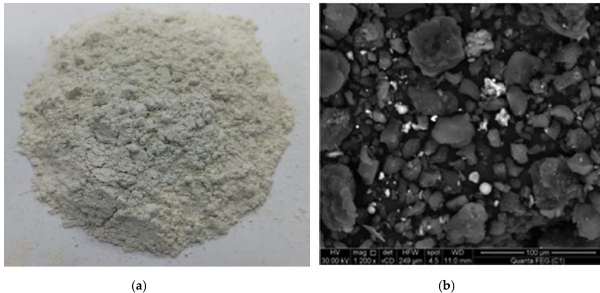
Figure 1. (a) Precipitated Calcium Carbonate (PCC) in powder form; (b) Microstructure of PCC [15].
