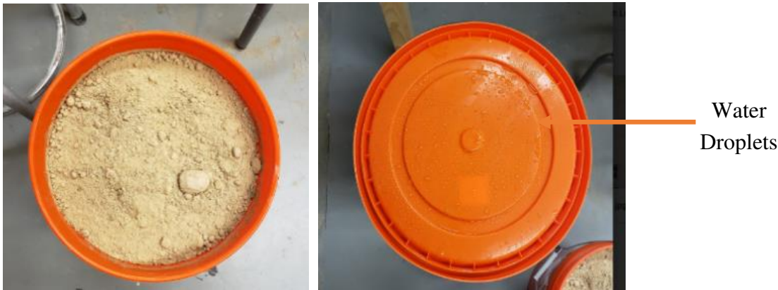
Figure 6. (a) PCC Samples; (b) Vapor in Bucket Lid.
