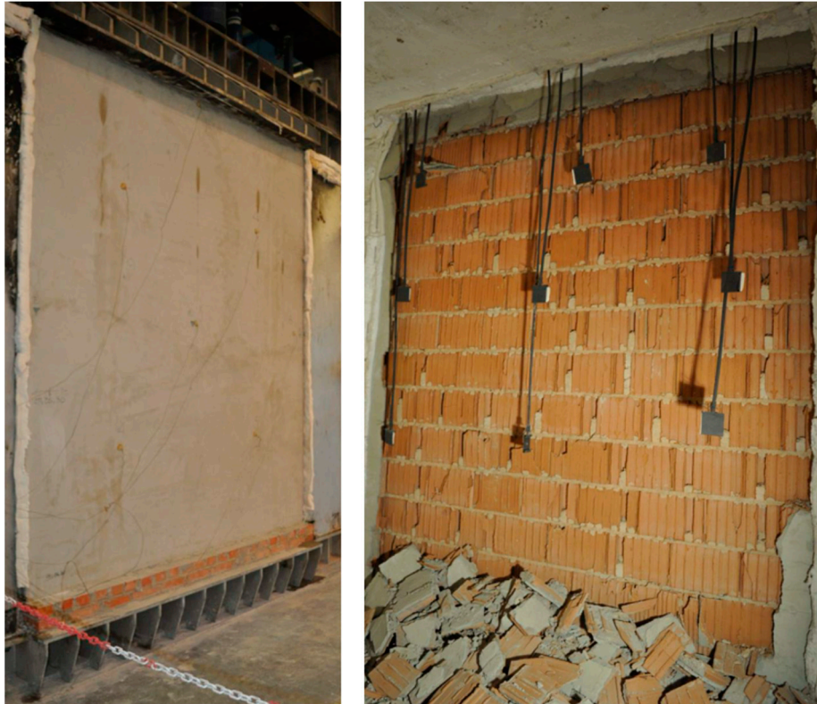
Figure 7. Post-test state – unheated side of the wall (on the left) and the heated side of the wall (on the right).
