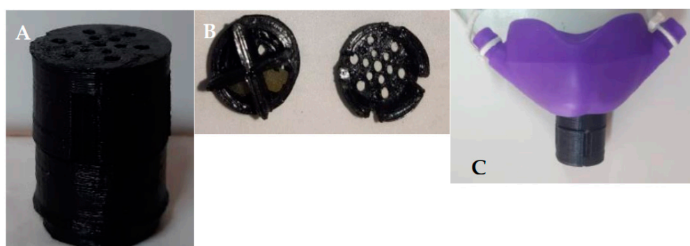
Figure 1. Modified nasal nitrous oxide mask; A: 3D printed box, B: Top and Bottom cover of the box, and C: Final shape of the box and the nasal mask.
