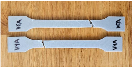
Figure 13. PLA tensile specimens printed with hexagonal infill (30 % density) after tensile testing: (a) unexposed sample (V1A), (b) sample after 7 days of exposure to mineral motor oil (V6A).
