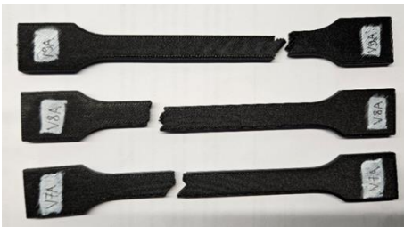
Figure 18. PLA+CF tensile specimens printed with different infill geometries: hexagonal (V7A), triangular (V8A), and linear (V9A), all with 30 % infill density. The fracture surfaces reveal geometry-dependent differences in filament failure and fiber–matrix interaction.
