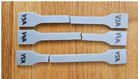
Figure 8. PLA tensile specimens printed with different infill densities: (a) 30 %, (b) 60 %, and (c) 100 %. Increasing infill density reduces the internal void fraction and produces a more compact structure.
