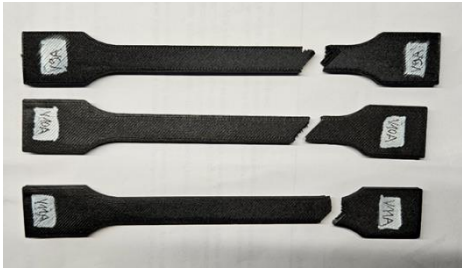
Figure 23. PLA+CF tensile specimens printed with different infill densities: (a) 30 %, (b) 60 %, and (c) 100 %. The increase in infill density reduces void size and enhances filament packing compactness.
