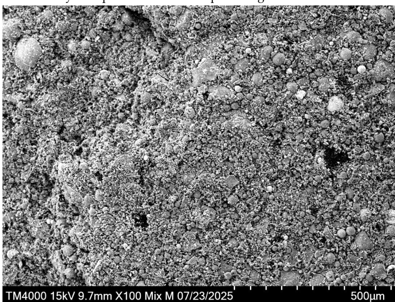
Figure 4. SEM micrograph of unactivated fly ash particles (100×).
