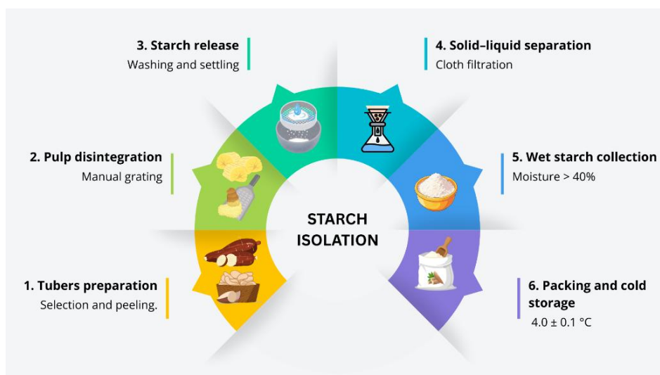
Figure 2. Simplified schematic representation of the starch isolation process from cassava.
