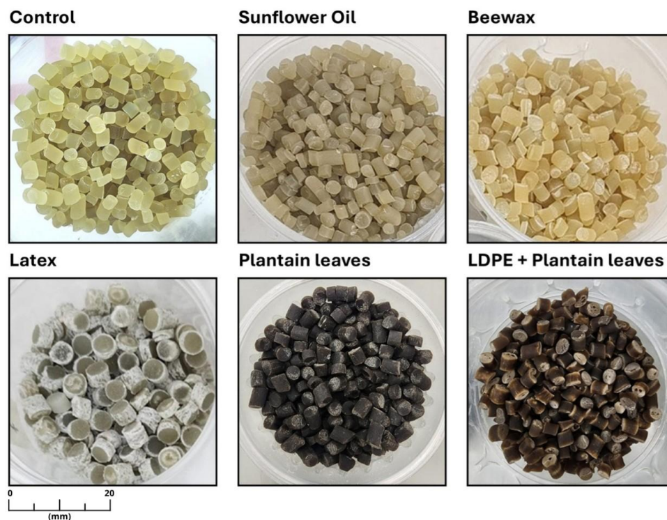
Figure 4. Pellets obtained from the extrusion of different compounded TPS formulations. All images are shown at the same scale; the scale bar represents 20 mm.
