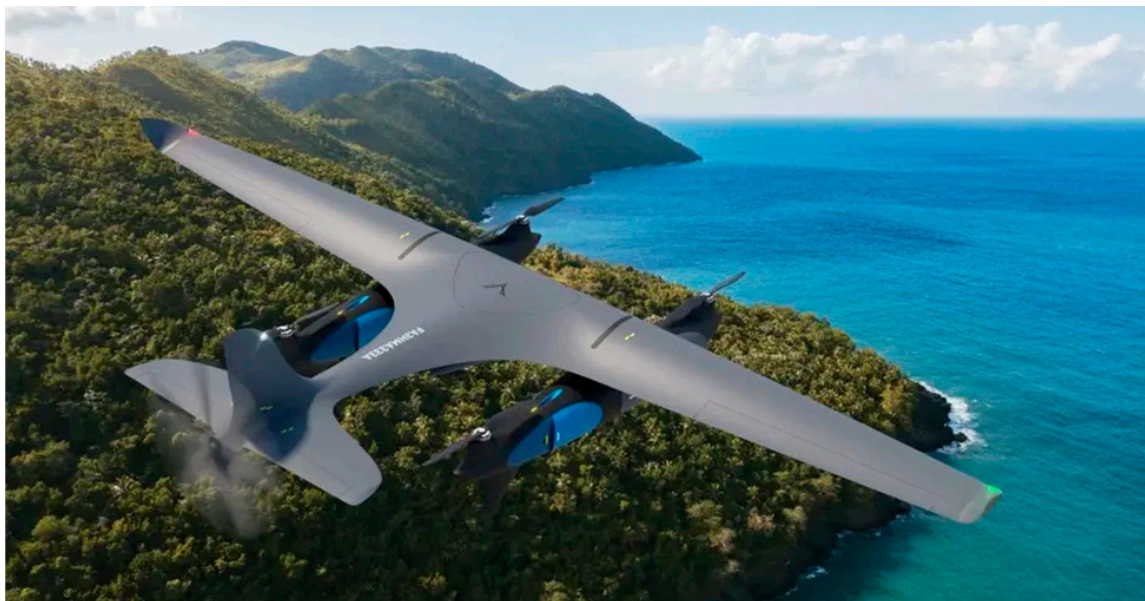
Figure 2. Raider, a fixed-wing hydrogen-powered drone. Credit: Heven Drones.
