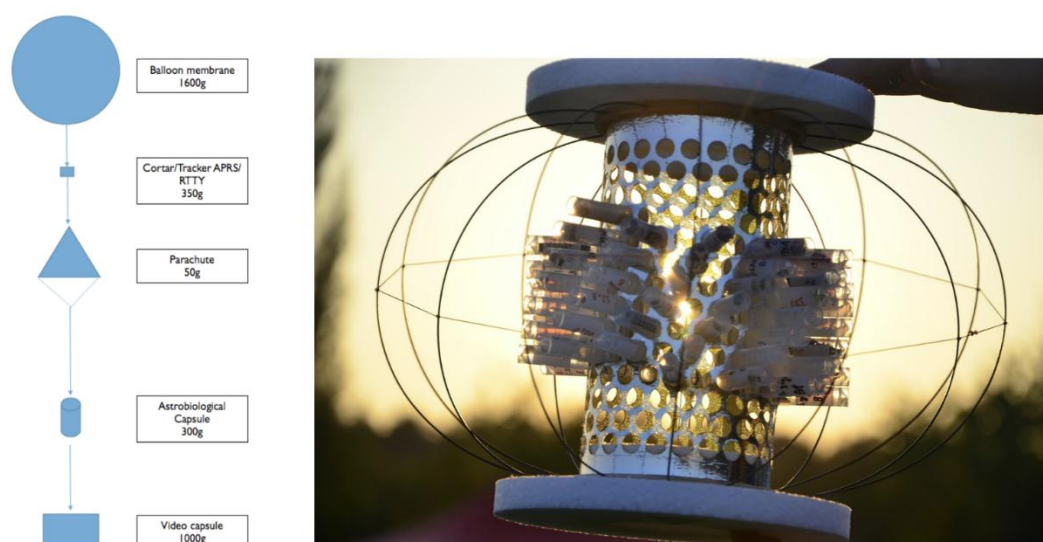
Figure 1. The following diagram illustrates the high-altitude balloon assembly for two flights of the stratospheric mission. During the nocturnal flight, the video capsule was detached, thereby reducing the payload mass and enabling the attainment of greater altitude. The astrobiological capsule has been designed with the objective of being ultralight, with the capacity to expose more than 200 biological samples in 2ml testing eppendorfs.
